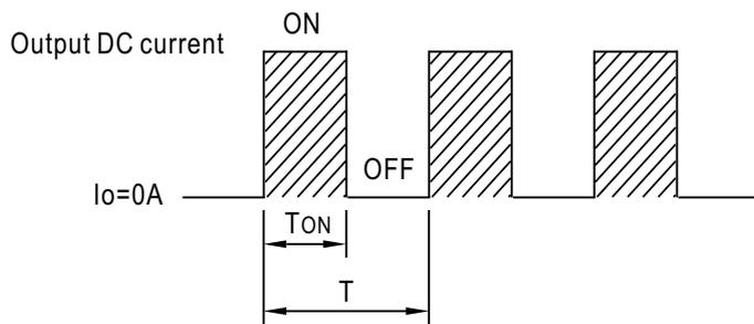
$$\text{Duty cycle(\%)} = \frac{T_{ON}}{T} \times 100\%$$
