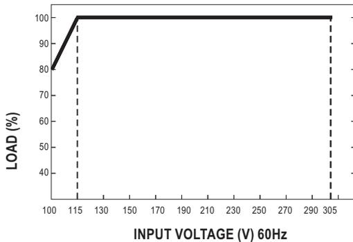
※ De-rating is needed under low input voltage.
